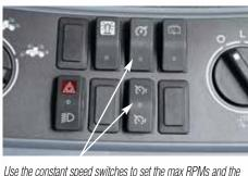
Use the constant speed switches to set the max RPMs and the speed adjustment switch or throttle to return engine speed to the desired level after making a turn.
